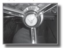
Pull off the center of the steering wheel.
