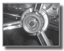
Thread the bolts of a steering wheel puller into the threaded holes. Use the correct bolts. Turn the center bolt of the puller to pop the steering wheel off. Remove the spring under the steering wheel.
