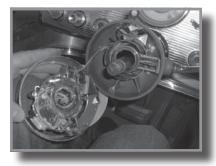
Pull forward the chrome shift indicator flange. Be careful not to lose the two square head bolts which held down the chrome shift flange. The detent plate is seen here on the chrome flange plate at 7 o'clock. Remove the two screws holding down the detent plate and remove the detent plate.
