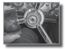
Scribe with a screwdriver or awl a mark towards the hole on the deep dish washer, so you will know in what position to reinstall the steering wheel.
