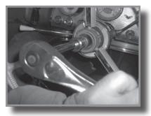
Upon removing the nut and the deep dish washer you will find two threaded holes on either side of the center threaded rod.
