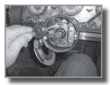
Remove the nuts at 11 o' clock and 5 o'clock. Unscrew the turn signal electrical switch.
