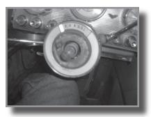
Remove the screws at 9 o' clock and 1 o' clock holding the plastic shift indicator. Lift off the plastic piece from the bottom.
