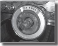
Reinstall the pieces in the reverse order. One tip on reinstallation: put in the square head bolts into the chrome shift flange and then thread on the nuts a few threads. This will help prevent you from losing your mind when the bolts fall off into the shift column.
