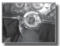
The plastic shift indicator will remain attached by the horn wire. Unscrew and remove the turn signal lever. Remove the spring on the turn signal switch with a small screwdriver. Keep one finder over the spring to prevent it from becoming a projectile. Pull out the plate assembly for the turn signal switch (It connects the turn signal lever to the turn signal electrical switch
